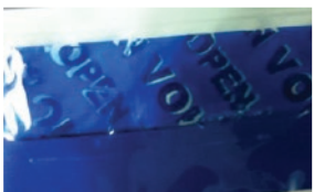
Result after being torn in ambient temperature
